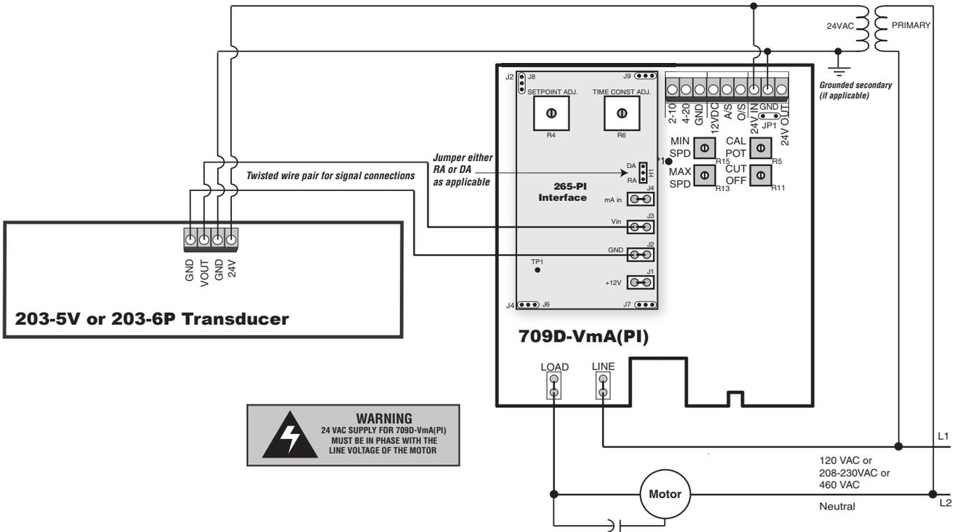
Wiring diagram for 709D-VmA(PI) & 203 Series Transducers
