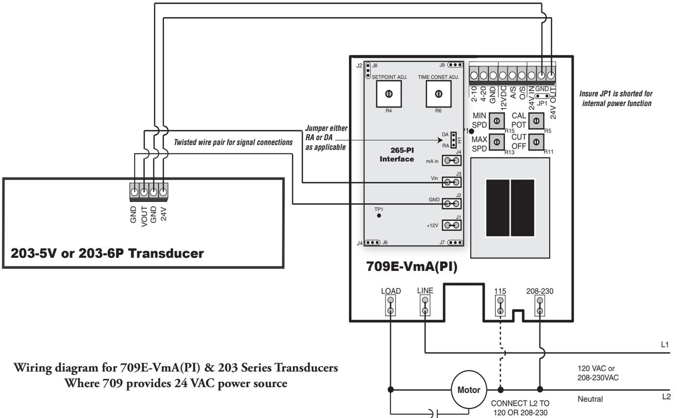
Wiring diagram for 709E-VmA(PI) & 203 Series Transducers
