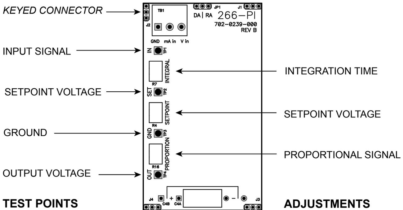
Figure 2 - Test Points & Adjustments
