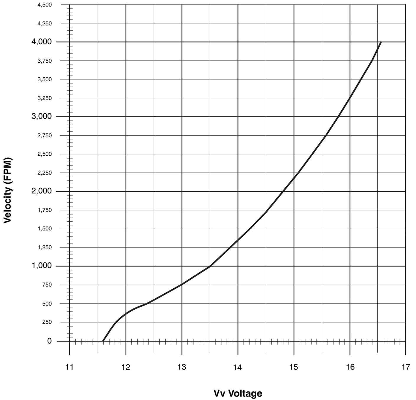
Velocity (FPM) vs. Velocity Volts
