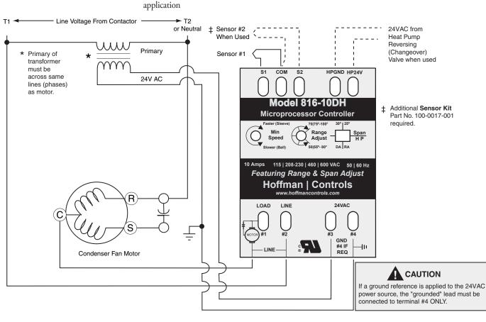
Wiring Diagram for the 816-10DH Figure 1
